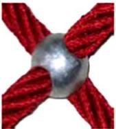
**BALL KNOTS** This will be a one-piece compressed aluminum ball, compressed in place with 150,000 pounds force (667 kN) to prevent the connection from moving and causing premature cable wear.
